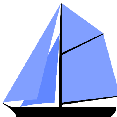
Figure 2. A schematic depiction of a cutter rigged sailing vessel, with a bow sprit projecting forward of the bow. Note the fore and aft arrangement of all sails. (Image: Casito at Wikipedia: https://commons.wikimedia.org/wiki/File:Sail_plan_cutter.svg ).
